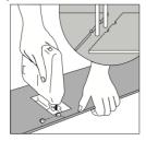
**8. Door molding and skirting:** Lay a board (with the decorative side down) next to the door molding and saw as shown in the figure. Then slide the floorboard under the molding.
