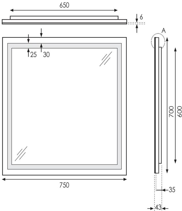
Note: This product must be installed with a minimum distance of 150mm between the infrared sensor and an adjacent countertop or obstruction to ensure correct function of the sensor. The IR sensor will not function correctly without this clearance.
