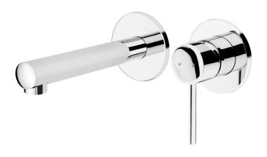
Brushed Nickel (PVD) COLOUR/FINISHES Brushed Brass (PVD) Matte Black Chrome PRESSURE TYPE All Pressures 35kPa MIN. PRESSURE 500kPa (As per NZ Building Code AS/NZ MAX. PRESSURE 3500.1) WELS RATING Low/Unequal 3 Star; 8L/min Mains 4 Star; 7.5L/min 65°C MAX. TEMPERATURE PLUMBING CONNECTION 15mm FACEPLATE DIAMETER 80mm
