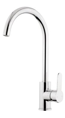
PUR11CH PRODUCT CODE FEATURES Cold Start Technology Brushed Brass (PVD) COLOUR/FINISHES Brushed Gunmetal (PVD) Matte Black Chrome All Pressures PRESSURE TYPE MIN. PRESSURE 35kPa MAX. PRESSURE 500kPa (As per NZ Building Code AS/NZ 3500.1) WELS RATING Low/Unequal 5 Star; 5.5L/min Mains 4 Star; 7L/min MAX. TEMPERATURE 65°C 15mm PLUMBING CONNECTION
