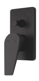
NRT35BK PRODUCT CODE Brushed Nickel (PVD) COLOUR/FINISHES Brushed Brass (PVD) Brushed Gunmetal (PVD) **Matte Black** Chrome PRESSURE TYPE Mains Pressure only MIN. PRESSURE 150kPa 500kPa (As per NZ Building Code AS/NZ MAX. PRESSURE 3500.1) 65°C MAX. TEMPERATURE PLUMBING CONNECTION 15mm FACEPLATE (W X H) 90 x 160 mm
