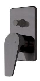
NRT35BG PRODUCT CODE Brushed Nickel (PVD) COLOUR/FINISHES Brushed Brass (PVD) **Brushed Gunmetal (PVD)** Matte Black Chrome PRESSURE TYPE Mains Pressure only MIN. PRESSURE 150kPa 500kPa (As per NZ Building Code AS/NZ MAX. PRESSURE 3500.1) 65°C MAX. TEMPERATURE PLUMBING CONNECTION 15mm FACEPLATE (W X H) 90 x 160 mm
