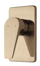
NRT30BB PRODUCT CODE **Brushed Brass (PVD)** COLOUR/FINISHES Brushed Gunmetal (PVD) Matte Black Chrome PRESSURE TYPE All Pressures 35kPa MIN. PRESSURE 500kPa (As per NZ Building Code AS/NZ MAX. PRESSURE 3500.1) 65°C MAX. TEMPERATURE PLUMBING CONNECTION 15mm FACEPLATE (W X H) 90 x 160 mm Watermark CERTIFICATION
