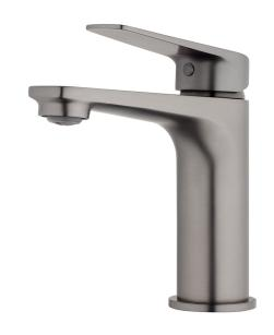
NRT20BG PRODUCT CODE Brushed Brass (PVD) COLOUR/FINISHES **Brushed Gunmetal (PVD)** Matte Black Chrome PRESSURE TYPE All Pressures MIN. PRESSURE 35kPa MAX. PRESSURE 500kPa (As per NZ Building Code AS/NZ 3500.1) **WELS RATING** Low/Unequal 3 Star; 8L/min Mains 4 Star; 7.5L/min MAX. TEMPERATURE 65°C PLUMBING CONNECTION 15mm CERTIFICATION Watermark SPOUT HEIGHT 108mm SPOUT REACH 120mm REPLACEMENT PART/S FORPT299 - 35mm North Basin Cartridge
